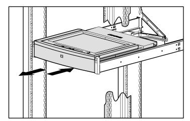
Figure 2-12. Accessing the monitor
